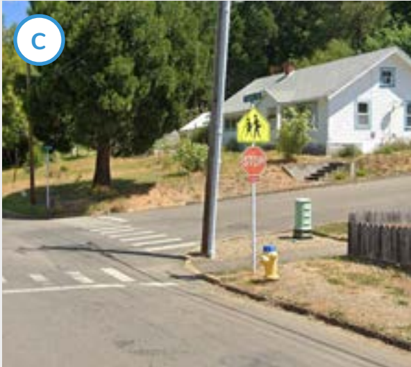
Throughout the City of Drain, stop signs and school crossing signs are being combined on one signpost. Location: East B Avenue and North Main Street intersection.
