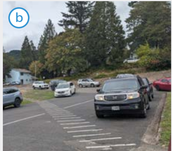
The two diagonal crosswalks leading to the school's main entrance are both poorly marked and small. The diagonal sidewalk results in irregular vehicle stopping behavior to avoid the crosswalk. Location: East B Avenue.
