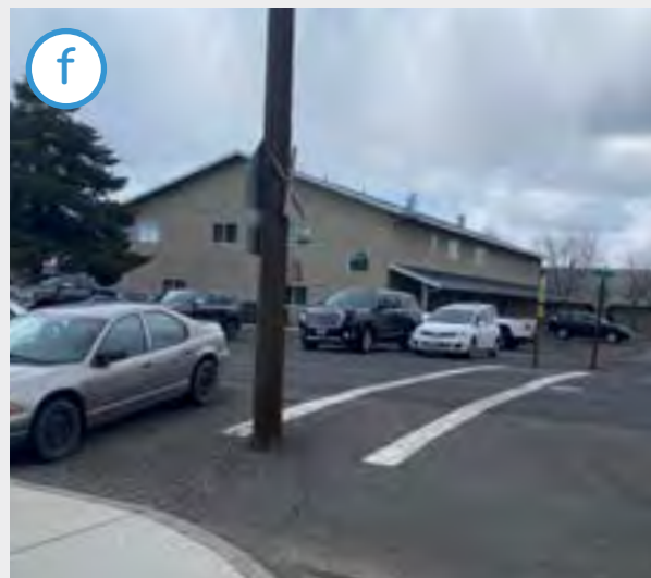
This photo shows the standard crosswalk to the east of the school entrance (also shown in photo a) with a utility pole the middle of the striping where students cross and enter the sidewalk.
