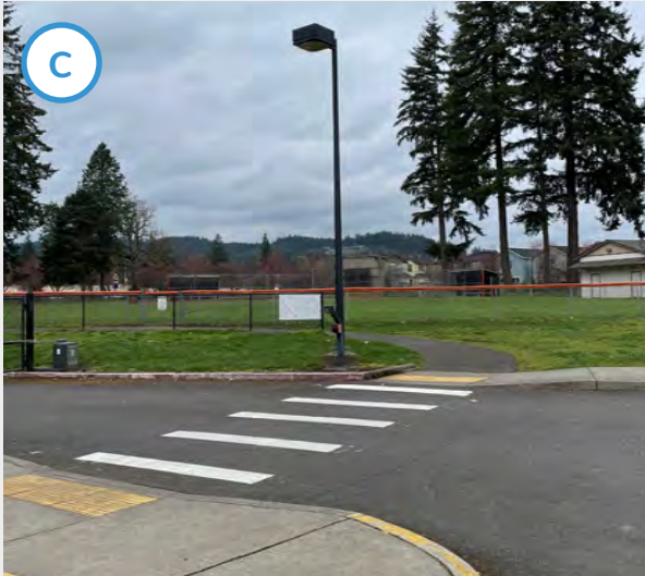
There is a marked crosswalk to the west of the entrance of the school crossing the bus access road. Like other locations in Scappoose, the crosswalk width here may be below an ideal width.
