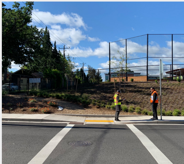
The existing crosswalk at May St and 9th St could use enhancement and emphasis to increase visibility, such as warning signs. Cars parked too close to the crosswalk on the east side also reduce sight lines.
