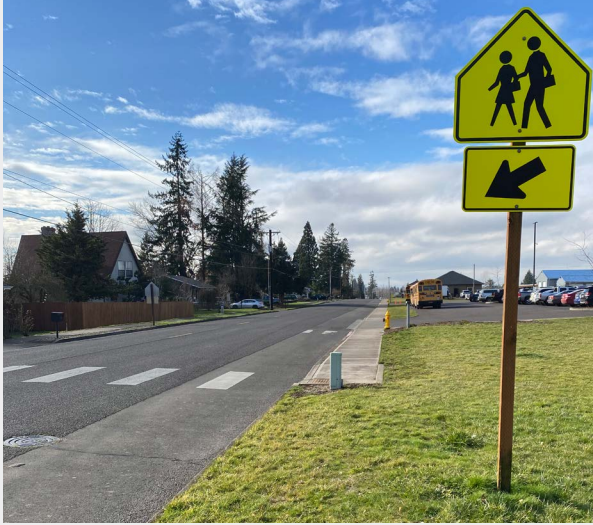
The crossing and signage on Marquam St east of the high school are not highly visible to drivers who frequently speed in the area. There is a need for traffic calming measures and/or crosswalk enhancement and improved lighting.
