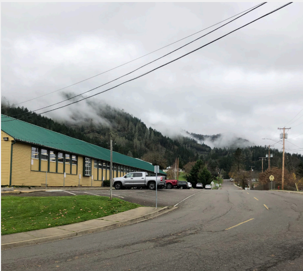
The sharp turn between Rice St and Spruce Ave creates a challenging environment for students walking and biking because vehicles are unable to see students on the crosswalk until they've rounded the corner. A single flashing beacon on the south end of the parking lot serves as some warning, but improvements can be made for the Rice St crosswalk. Also note that there is no separation for pedestrians between the parking lot and the general travel lane on Spruce Ave.
